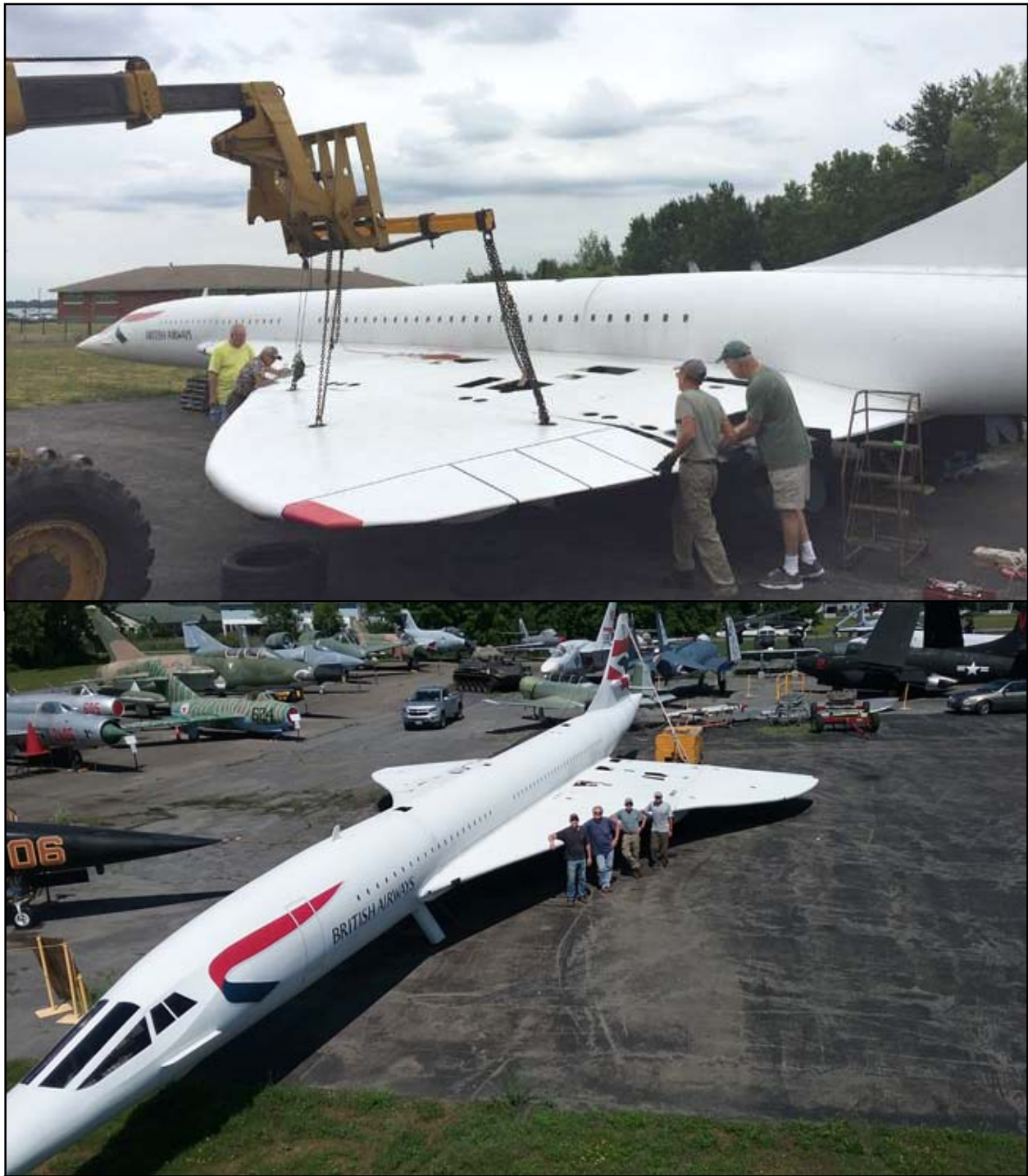
Above Top: A Restoration crew reinstalls the Concorde's left wing tip. Pictured from right to left are Restoration Group volunteers Mike Cole, Dan D'Amour, Dave Tripp and Peter Bergendahl. Not pictured is Rich Bievenue who is operating the forklift.
